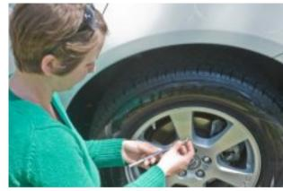
and before long road trips, perform this DIY routine: check tire pressure, check tread depth, check the overall condition of the tires for cuts, cracks, splits, punctures, irregular wear and bulges.
