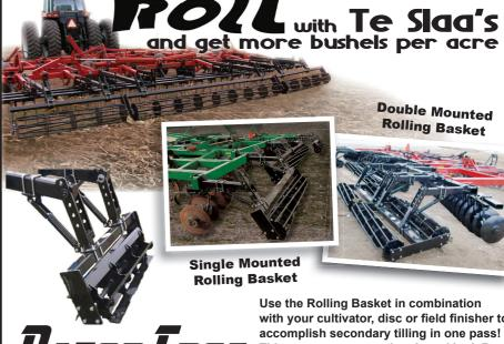
with your cultivator, disc or field finisher to accomplish secondary tilling in one pass! This creates an exceptional seed bed. By creating downward pressure it reduces clod size, improves the ecenness of your seed bed, and knocks dirt off of old root crowns and any existing weeds.
