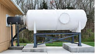
laser awarded to UTSI by the Office of Naval Research. So just how big is one of academia's largest wind tunnels? The test section measures in at 24 inches by 24 inches, making it 60 percent of the size of AEDC's Mach 1.5 to Mach 5.5 facility. When the tunnel is operated, air flows due to a vacuum created in a large tank outside the building. The 105-foot tube at the opposite end holds pressurized air that rushes through the nozzle and test area when a diaphragm is ruptured.
