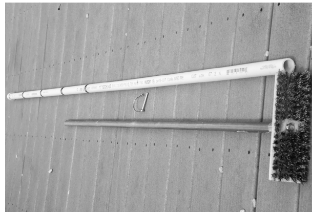
Homemade 3-in-1 thingy. It’s a deck brush, a pusher-offer, and a depth gauge.
