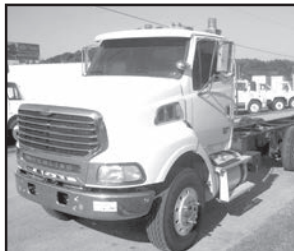
09 STERLING AT9500 C&C, 218 K MILES, 556 VW MERCEDES ENG., 10 SPD., TANDEM, 232" CAB TO AXLE, AIR SUSP., A.C., P.S., DOUBLE FRAME, 4:11 GEARS, STK# 7365
