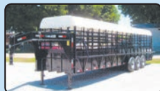
J&R GVW21K 6'x16 thru 6'x36 3 ax., 3 brakes, pipeside
