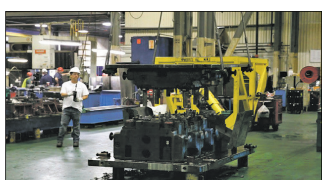
An employee at the Toyotetsu plant in Somerset, Kentucky, uses a crane to open a stamping die for repair in the die maintenance department. [COURTESY PHOTO]
