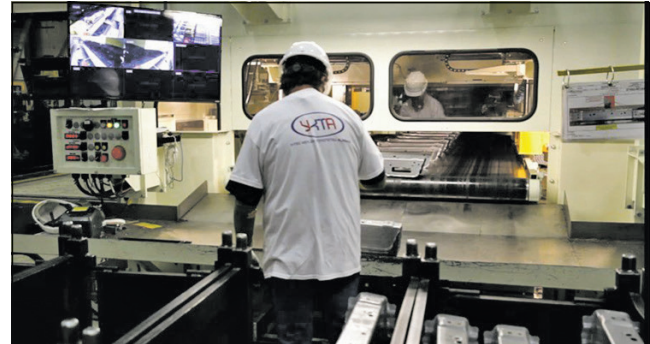
An employee at the Toyotetsu plant in Somerset, Kentucky, operates a stamping press and performs quality checks and packing of metal auto parts. [COURTESY PHOTO]
