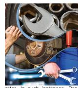
rotor. In such instances, Pep Boys® recommends replacing the brake pads immediately. If the grinding noise is audible while the vehicle is in motion, debris might be stuck inside the brakes. Drivers might be able to dislodge this debris by repeatedly moving their cars forward and backward in a safe place, such as a driveway. If that does not work, have the brakes serviced by a qualified mechanic.
