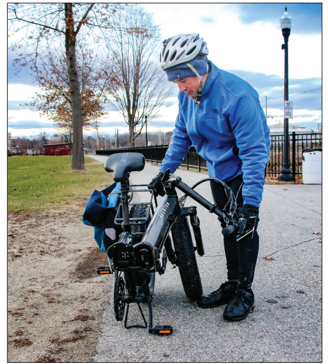
Nate LeClair’s Aventon Sinch ebike is folded for transport in his car. The bike is battery-powered with a range of 40 miles in throttle mode, and folds for storage or transport. (Tsukroff photo)
