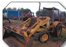
Case 480ELL - 4 cyl. Cummings engine, has 3pt w/hyd. side link for tilt & hyd. toplink $6,850
