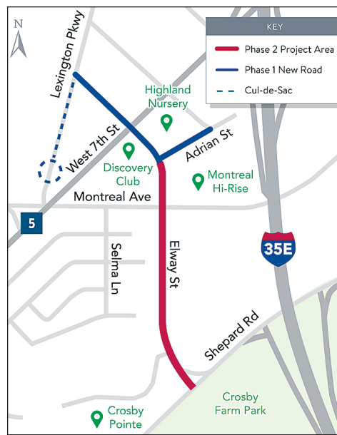
The second phase of construction will extend Lexington Parkway through county right-of-way and along Elway Street to connect with Shepard Road.
