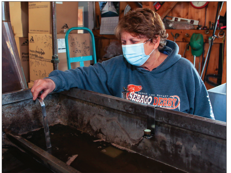
Jo Hartwell, the owner of Jo's Sugarhouse on Sebago Lake Road on the north end of Gorham, checks the drain plug on the evaporator used to boil down maple sap to make maple syrup. It takes more than 40 gallons of sap to make a gallon of syrup. (Tsukroff photo)
