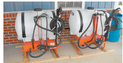
800-3ph-55 gal. sprayer w/Hamilton boomless nozzle, hand wand and delavan pump, NEW $995.00
