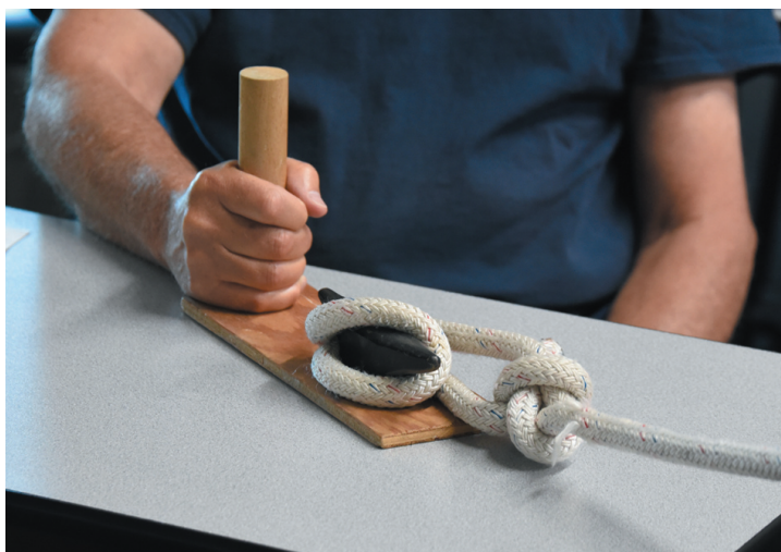
Here is loop made with a bowline knot and used to secure a line to a cleat that is too small for the line's large diameter.
