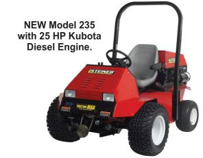
Fully hydrostatic unit. Front-wheel drive, rear-wheel steer. Foot pedal for F&R. Unit accepts many of the "Quick Hitch" front mounted "Steiner" attachments.
