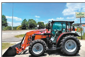
MF 4707 - 70 hp turbo diesel, 12-speed power shuttle transmission, 2 hyd remotes, NO DEF and NO REGEN SYSTEM, Deluxe Cab Call for Pricing
