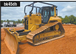
2018 CATERPILLAR D6N LGP EROPS, S/N: CAT00D6NKS GG00279, 6 Way Blade, Rear Screen, Grade Control, Diff Steer $174,900
