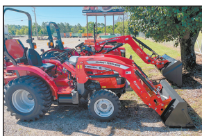
MF 1835E - 4WD, quick attach loader, shuttle shift, 36 HP with turbo Call for Info & Pricing
