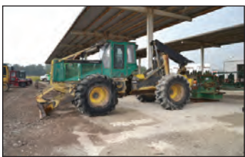
TIMBERJACK 460D DA GRAPPLE SKIDDER
