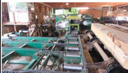
Brewco B1600 Grade Resaw w/Complete Runaround, Cab & Computerized Controls
