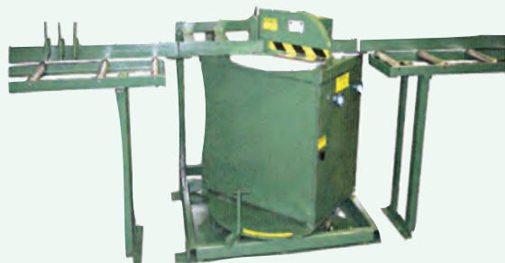
ANGLE CHOP SAW Cuts 0° to 45° on a 2x8 and 0° to 40° on a 2x10 Fast Cycle
