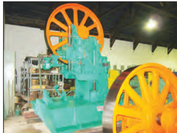
Salem 6Ft. Air Strain Bandmill
