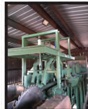
CHAIN SCRAGGS FOR SMALLER LOGS Add an Edger for a finished cant
