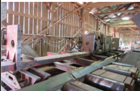
Lane Modular Sawmill w/Silvatech Setworks, 12" Slab Drop, 4 HB Carriage, 125hp Motor & Tyrone Berry 230 Carriage Drive
