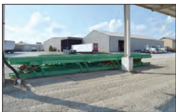
24INCH X 80FT VIBRATING CONVEYOR
