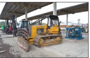
JOHN DEERE 550A DOZER WITH WINCH
