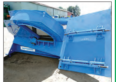
Acrowood 6120 Slant Disc Chipper
