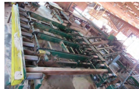
Lane Modular Sawmill w/Silvatech Setworks, 12" Slab Drop, 4 HB Carriage, 125hp Motor & Tyrone Berry 230 Carriage Drive
