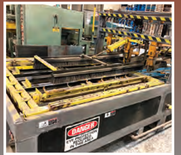
Senstar 3-stringer Pallet Nailer #2759
