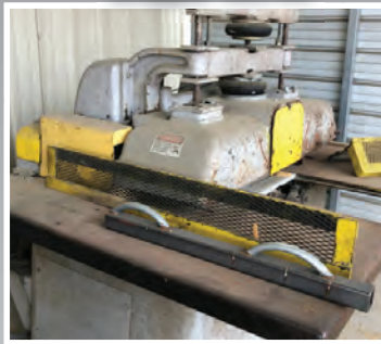
Diehl Straight Line Rip Saw #2758
