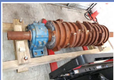
Montgomery 50PM-ER Rotor Assembly 10554
