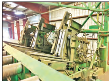
USNR 42In. Tilted LP Carriage
