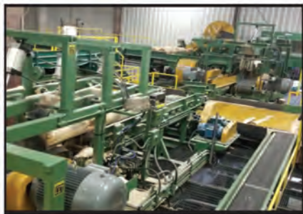
TANDEM SCRAGGS FOR LARGER LOGS Comes out a finished cant with one person
