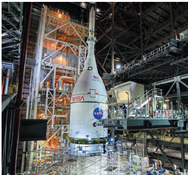
On October 21, the Orion Space Capsule was "stacked" on the SLS rocket, preparing for Artemis 1 launch in February, 2022.
