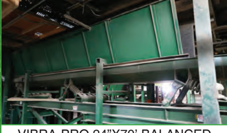
VIBRA-PRO 24"X70' BALANCED VIBRATORY CONVEYOR
