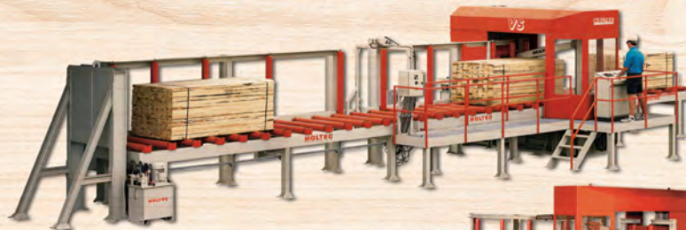
AUTOCUT® High-Volume Automated Crosscutting with programmable PLC Controls
