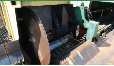
60" INSERT TOOTH WHOLE LOG CUT OFF SAW
