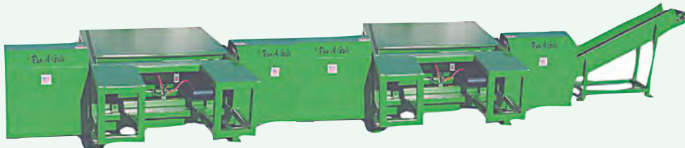
The RUN-A-GADE Bandsaw Pallet Disassembly System
