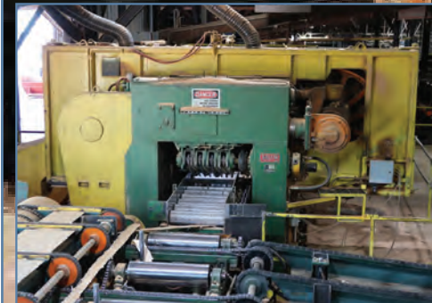
SALEM 5' TWIN HORIZONTAL BAND TEMPOSONIC POSITIONED RESAW
