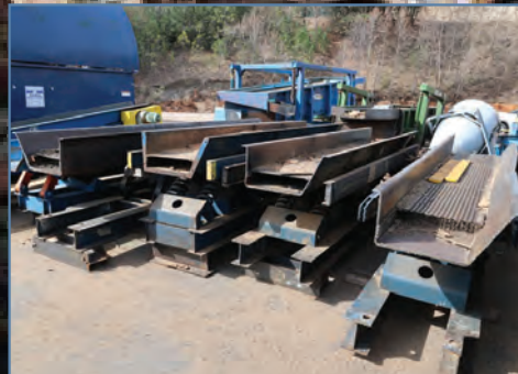
MILLPOWER APPROX. 18"X42" BALANCED VIBRATORY CONVEYOR
