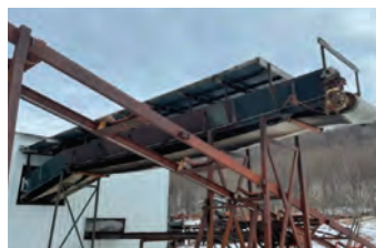
52" X 84' Inclined Belt Conveyor, Bed pan approximately 15 feet high off the ground
