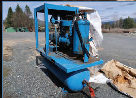
QUINCY MG SERIES 30 HP ROTARY SCREW COMPRESSOR
