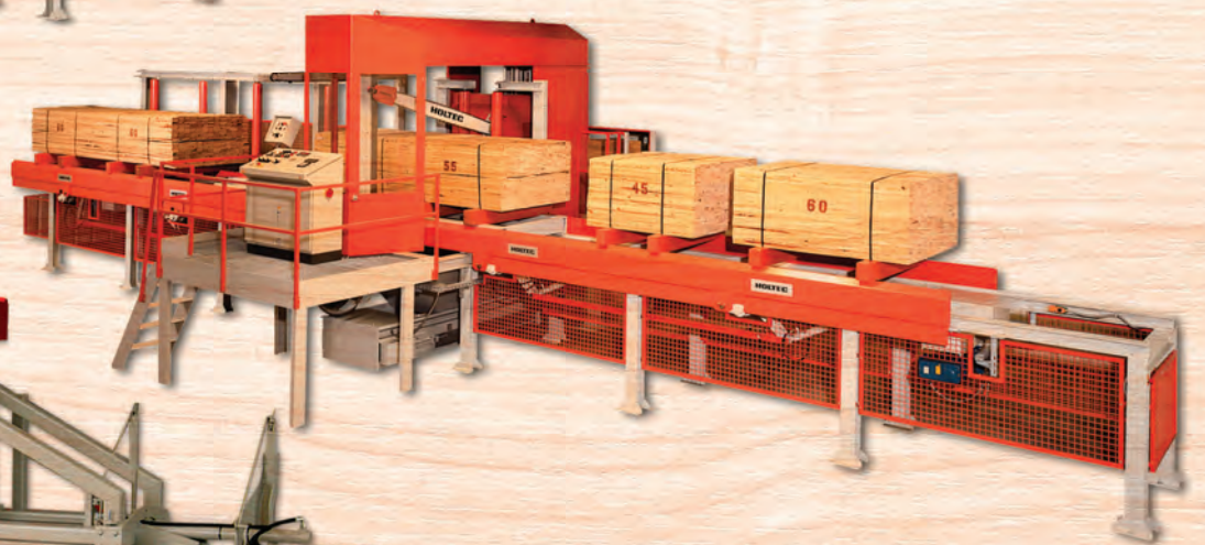
SELECUT ® High-Volume PET and Market Premium Length Crosscutting with Integrated Power Package Squeeze
