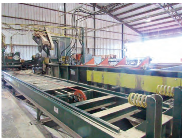
Pioneer 2 HD Modular Mill w/ Top Saw and Computerized Controls
