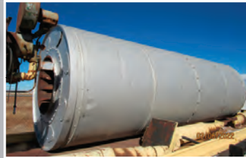
8'x30' Drum Dryer Gas Fired
