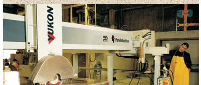
W.R. Watson's State-of-the-Art Granite & Quartz Fabrication Plant Utilizes Computerized Saws, Edge Profilers, Crane and Vacuum Lifts
