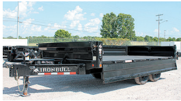
Deck Over Drop Sides Dump Trailers
