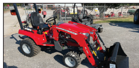
MF GC 1723e Tractor 24 hp Diesel engine, hydrostatic transmission, quick attach loader, CAT 0 3 point hitch, power steering, mid-PTO for mid mount attachments. Call for Best Price
