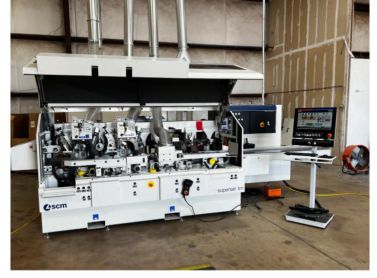
planers and saws plus four custom 4, 5 & 6 head moulding machines that can produce boards and moulding up to 12" width.
