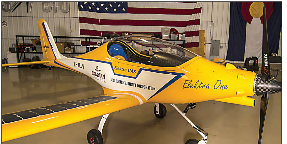
SUN FLYER: Single-seat technology demonstrator for the solar-electric Sun Flyer.
