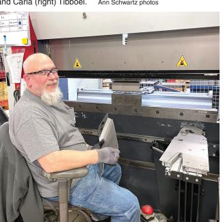
Noel Taylor of Crosby is a press brake operator with over 30 years of manufacturing experience. The machine he operates bends metal parts for Polaris Ranger doors.
