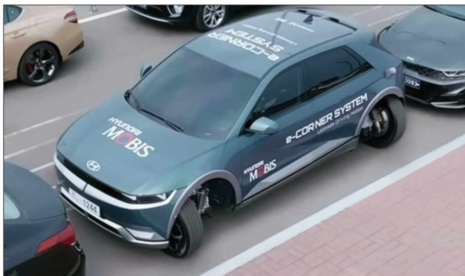
Hyundai's e-Corner System can turn all four wheels 90 degrees. (Hyundai)
