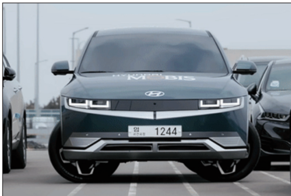
e-Corner System allows for a vehicle to move sideways. (Hyundai)
