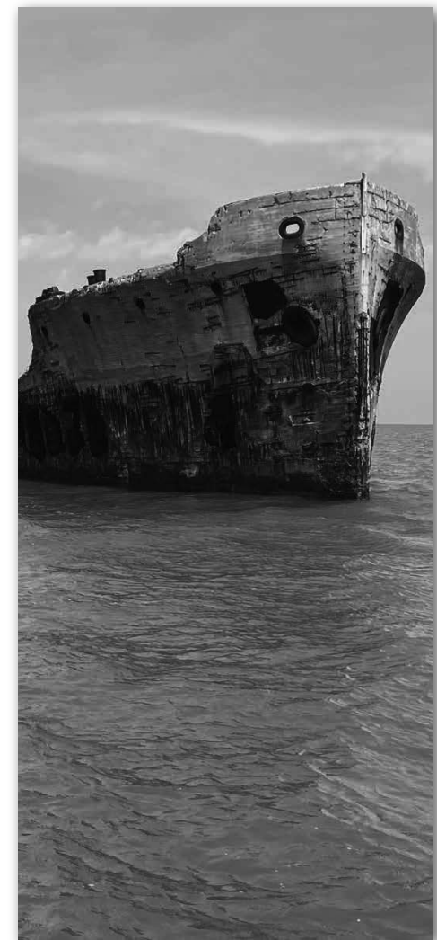
The SS Selma - a WWI tanker ship made entirely of concrete that was scuttled in shallow waters in Galveston Bay in 1920.
