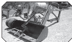
IH 2350 Loader - fits IH 66 thru 86 series, 7' bucket, no welds, Stk#6692 - $4,000
