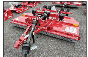
New 3510 - 10.5' pull type, 540 PTO, front chains $14,500
