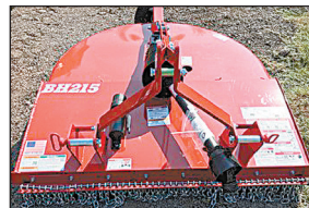
BH215 - 60", 3 pt, 540 PTO, 65 hp gear box, stump jumper, front chains - $3,650
