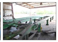
3-Strand log deck W/Stop & Loader. 10'6" X 40' Plus 4' Nose Skids. Hyd. Drive & Cylinder, Gearbox, H78 Chain.
