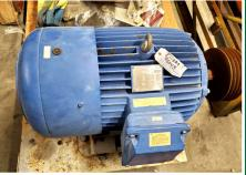
75hp 1778rpm TEFC Motor 10580.02
