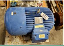
75hp 1778rpm TEFC Motor 10580.02
