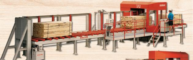
**High-Volume Precision Crosscutting** with Integrated Package Aligner and Loop Bander
