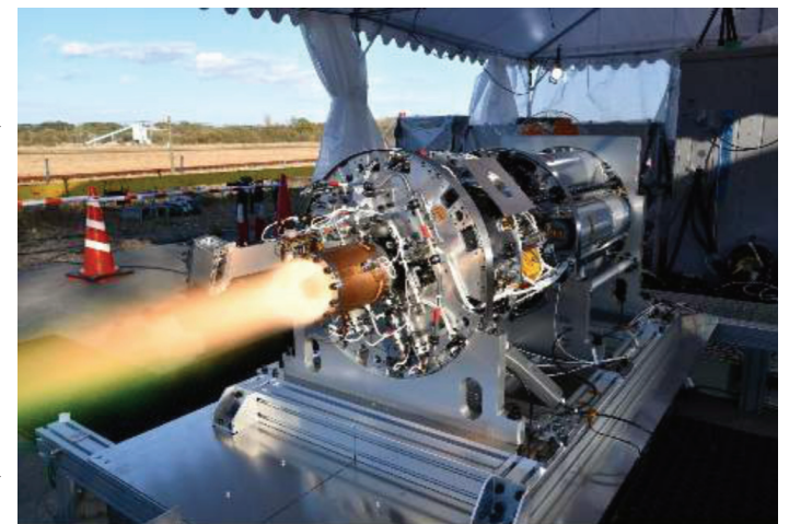
The rotating detonation rocket engine undergoes testing.
