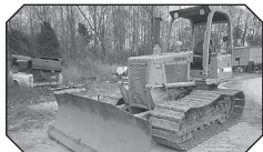
Dresser TD9H -1998, LGP, 70% U/C, Cummins 4 cyl. turbo diesel, runs good, Stk#6767- $21,500
