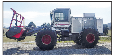
2013 Kershaw Klearway 500 3,210 hrs., Enclosed cab with AC, Heat; CAT 6.6 250 HP 6 CYL diesel engine; Articulating AHWI mulching head; 4x4; Rear winch; 70% rubber. "Always Serviced. Job Ready!" $98,500
