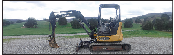
2017 John Deere 35G 6,519 hrs., Yanmar 24 HP diesel engine; 7,760 lbs operating weight; New sprockets; 50% tracks; 18" bucket; 4 way dozer blade; Long stick; Pattern control changer; Light package; Aux hydraulics; Original paint. "Serviced And Job Ready!" $19,500
