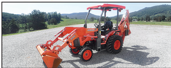
2016 Kubota B26 290 hrs., Kubota 24 HP DSL engine; 4,000 lbs operating weight; 4x4; 3 PT hitch and PTO; Hydrostatic transmission; Skid steer quick attach coupler bucket; Power steering; R4 Industrial tires. One Owner. Extra Nice! $23,800
