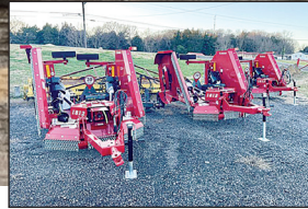
New 1812 Flex Wing Cutters 12', hyd. fold, 540 PTO $16,500
