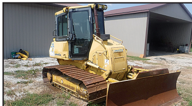
2011 Komatsu D39PX-22 6,646 hrs., Cab with A/C, Heat; 107 HP DSL engine; 21,800 lbs op weight; Good U/C; 6 Way blade; 3 forward 3 reverse powershift transmission; 21" steel tracks. Cranks And Runs. Has Electrical Problems $26,500
