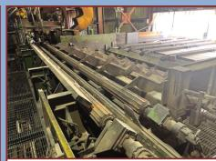
END DOG LINE FEEDER W/2024 USNR SCANNING & SOFTWARE
