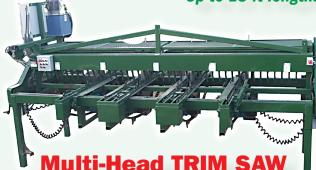
2, 3, 4 or 5 head models Adjustable heads with variable speed, chain feed drive motor w/starter
