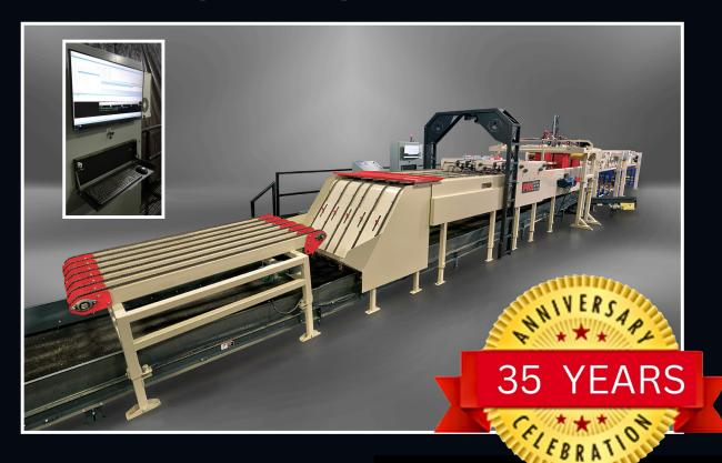
With only 1-2 operators, it feeds, seems, optimize output, cuts and sorts multiple lengths, widths **accurately and consistently at up to 3,600 boards per hour**
