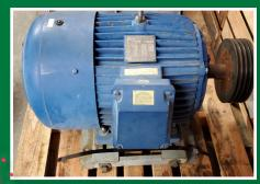
75hp 1778rpm TEFC Motor 10580.02
