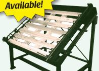
Assembles all size pallets (up to 50" x 50") with easy adjustments
