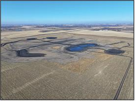
Landscape photo of early stages of wetland restoration work facing NW. Sediment removal can be seen already holding water and some tile removal lines are also visible, as well as embankment construction restoring the natural shoreline. Photo by Jake Chronister, Ducks Unlimited.
