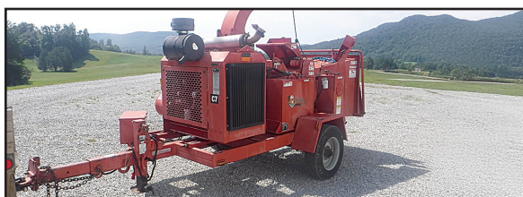
2011 Morbark Beaver M15R 1,872 hrs., JD 140 HP DSL engine; Auto speed; 15" inch max capacity; 9,000 lbs operating weight; Good tires; Pintle hitch; Original paint. $25,500
