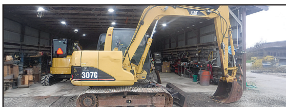
2006 CAT 307C 4,268 hrs., Cab with A/C, Heat; Good U/C; 34" Heavy duty bucket; 90" Dozer blade; 22 1/2" pads; Auxiliary hydraulics on boom. "Pre Def, Pre Emissions. Extra Nice!" $34,500
