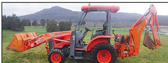
2013 Kubota L45 971 hrs., Kubota 45 HP 4 CYL diesel engine; Skid steer quick attach front loader bucket; Hydrostatic transmission; BT1000 Rear backhoe attachment; 540 PTO with 3 Point hitch; Wet disc brakes; Auxiliary hydraulics on rear boom; Original paint. "Pre Def, Pre Emissions. Nice Unit!" $26,500
