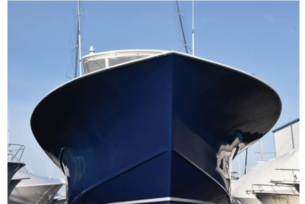
Fiberglass molding enables sleek lines and bow flare that are difficult to achieve in wood designs.
