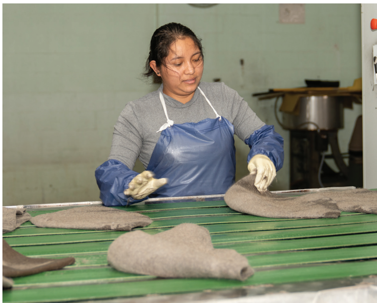
▲ This multi-roller machine only requires two workers as opposed to four workers for some of the others. Milken Yanes sorts and stacks hats ready to go to the next process.
