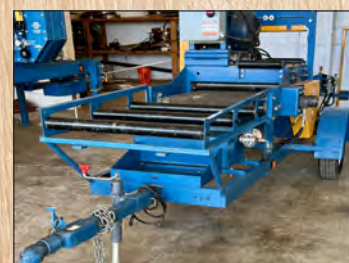
BAKER Model BE-O 24" wide 2-Saw Edger 15 HP on trailer
