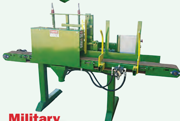
ANGLE CHOP SAW Cuts 0° to 45° on a 2x8 and 0° to 40° on a 2x10 Fast Cycle
