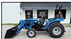
2025 LS MT232H, 32 hp, hydrostat trans., 4WD $27,500
