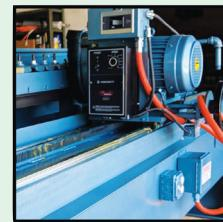
**GRINDING HEAD** - 5 HP Spindle Motor with Undervoltage Protection & Variable Speed Drive Control Box
