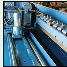
**CARRIAGE DRIVE** - Variable Speed DC Motor with Rack and Pinion Drive
