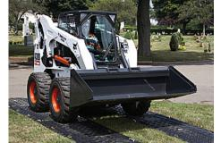
minating expensive ground restoration costs is why leading contractors specify AlturnaMATS. Simply lay these rugged 1/2" polyethylene ground protection mats end-to-end and you have an instant roadway or working platform...and you'll never get stuck again. AlturnaMATS handle 60-ton vehicles with ease. Available in sizes ranging to 4' x 8'. The good news, they eliminate soggy, splintered, warped, short-lived plywood.
