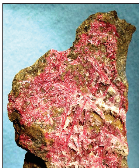
Cinnabar, the ore found at Almaden Quick Silver Mine that contains mercury
