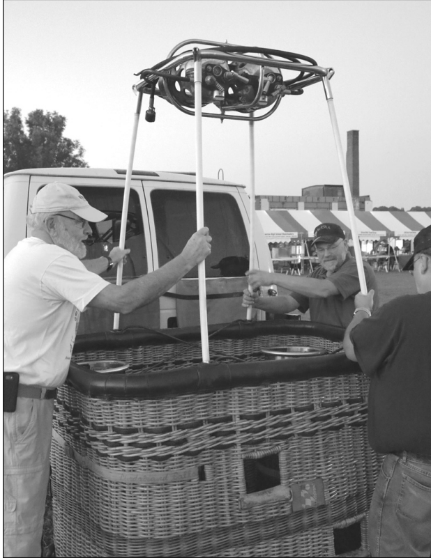
William Colyer (left) pilot of Last Penny out of Fairfield, CT, gets help from Ron Gravel and Ricky Wells to place the burner on the basket, on Friday morning. (Tsukroff photo)
