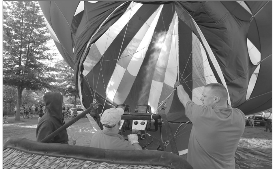
Crew members fire the burner to heat the air in the envelope of the Aerial Adventures balloon to bring it upright for lift off. (Tsukroff photo)
