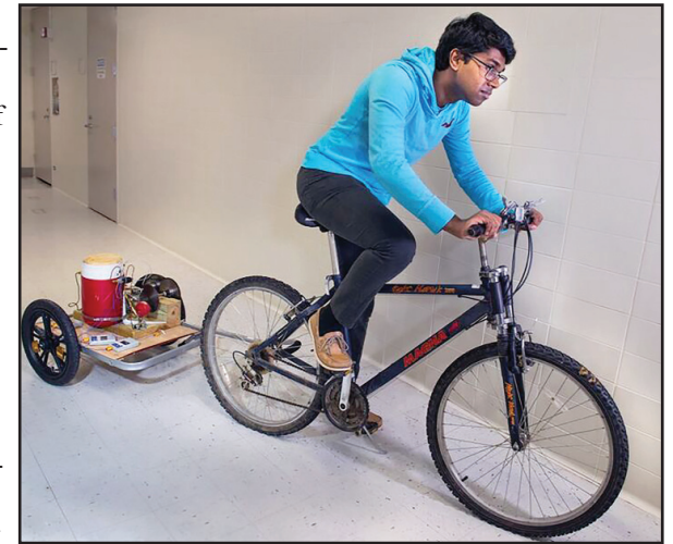
Sixteen-year-old Anurudh Ganesan from Clarksburg, Md. shows off his invention, the VAXXWAGON, a wheel-powered cooling system that keeps vaccines viable during the final stages of transport to remote locations. Courtesy Photo
