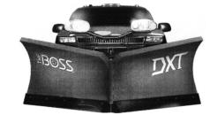
THE BOSS DXT combines both trip-edge and full moldboard trip technologies for high and low trip protection when striking hidden obstacles like frozen snow banks, manhole covers and curbs.
