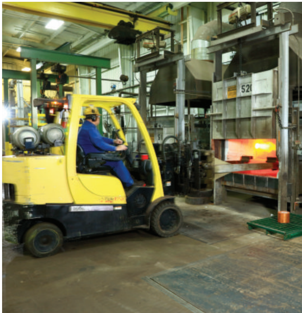
Above: A driver at Weldaloy is pulling a part that has just been heated so it can be taken to the hammer to be forged.
