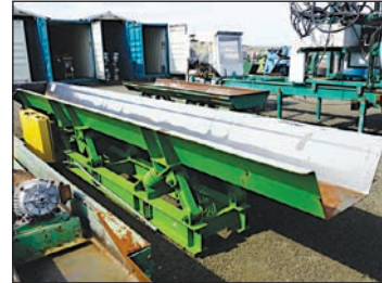
Mill Power Vibrating Conveyor
