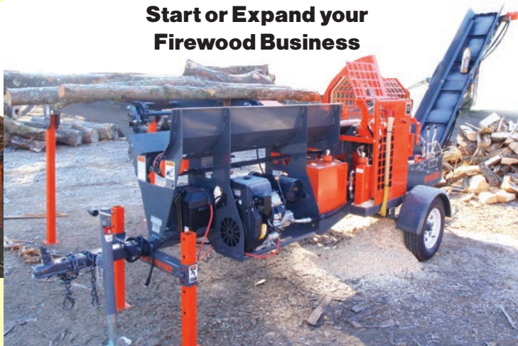
Model 1610EZ - Joystick control, gas or diesel, live deck or log lift, ultra mobile with integrated conveyor.
